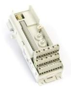
The TU811V1 is a 8 channel 250 V compact module termination unit (MTU) for the S800 I/O. The MTU is a passive unit used for connection of the field wiring to the I/O modules. It also contains a part of the ModuleBus.
